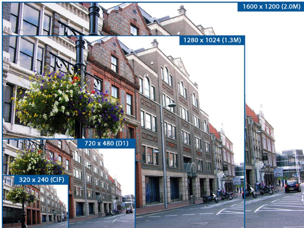
This is a comparison of different resolutions ranging from CIF to 2MP. Note how the 2MP size is at least 4 times larger than standard D1. A single Megapixel camera can replace multiple traditional cameras and they provide detail that is much more useful for identification.
