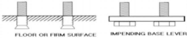
Step 2 fix the camera body on the floor or impending base level
