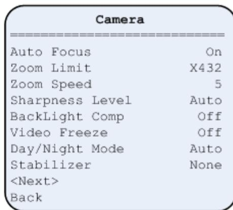
Note: The function of STABILIZER, Video Freeze will be only available when the camera has such functions. If the camera has, it can be set in the menu. If camera hasn't, None item will be showed in the menu, and can not be set.
